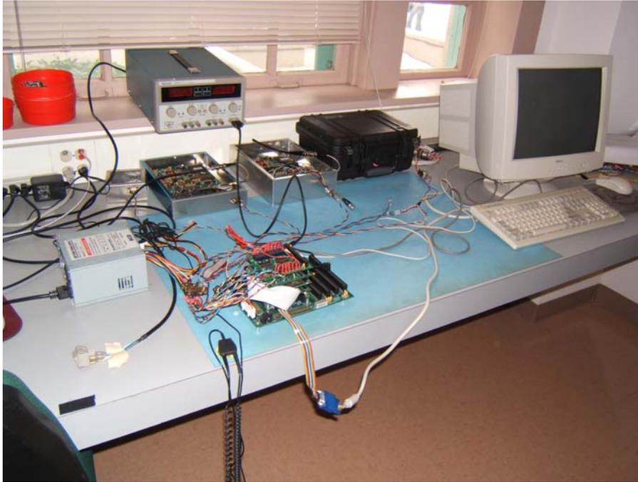
Nanosat “flatsat” lab for component testing
