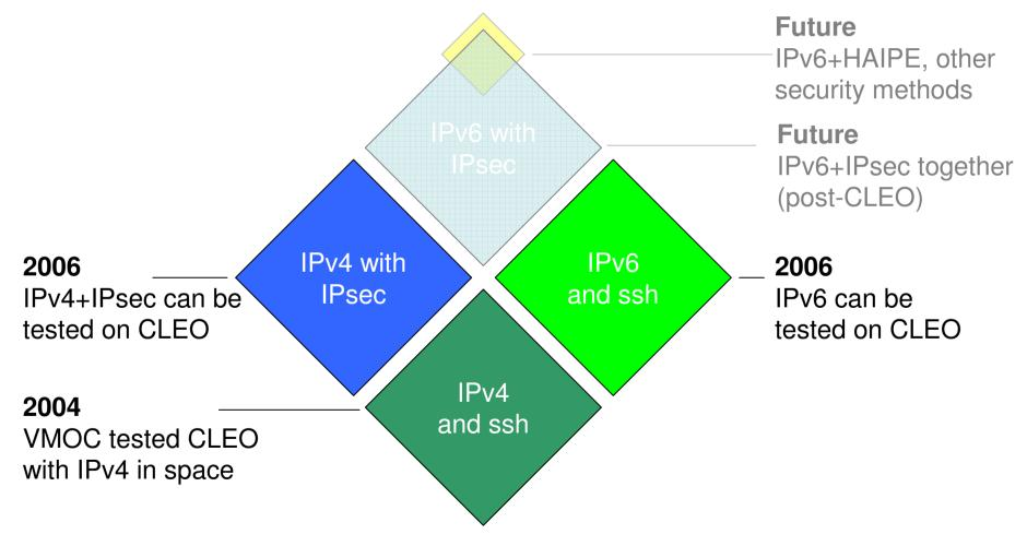
CLEO, the Cisco router in Low Earth Orbit, is able to show three of these five steps.
